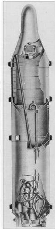
**Figure 6: SS-N-6 with the Submerged Engine**
